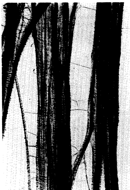
Figure 13 Typical micrograph of a drawn gel fibre, drawn at 117°C and subsequently washed at 114°C
